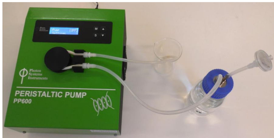
Fig. 6 Basic configuration of Peristaltic Pump.
