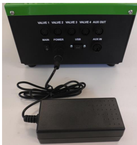
Fig. 7 Power cord connection of peristaltic pump.
