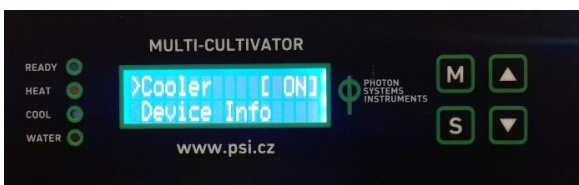
Fig. 3 MC 1000-OD front control display: Cooler ON.
