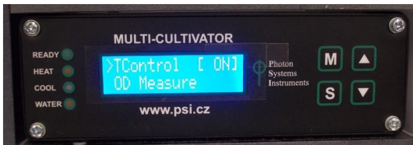
Fig. 3 Display of the MC 1000-OD control unit when Cooling Unit AC 710 is operating.
