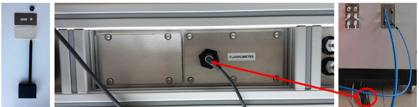
Fig. 21 Optical module installation.
