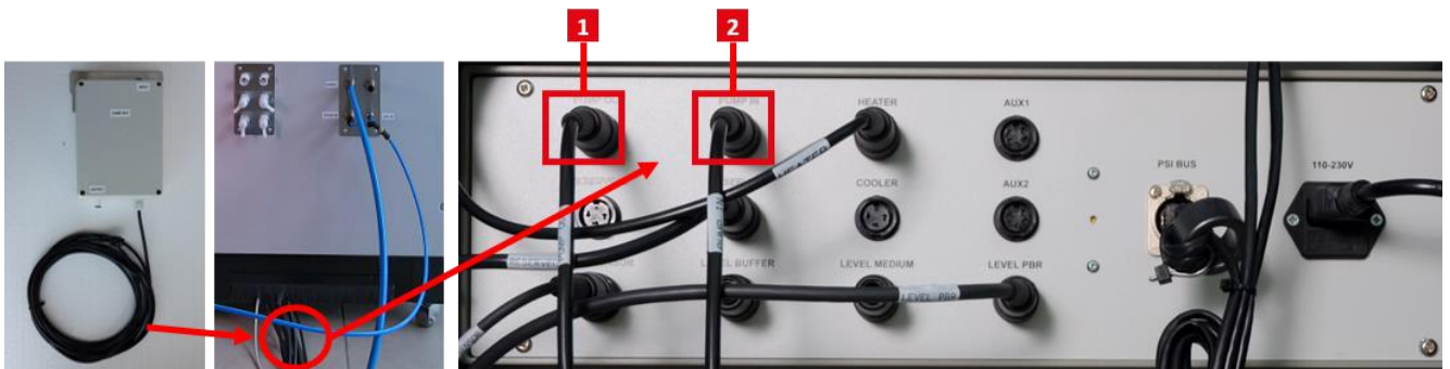
Fig. 30 Turbidostatic (diaphragm) pump installation.
